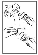
Push the roller (12) or paintbrush unit (13) onto the end of the handset with moderate force.
