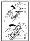
The roller assembly may now be dismantled into its three component parts; the roller (12), paint flow guide (11) and holder (10).
